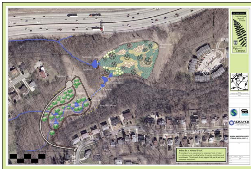
Top: Banklick Constructed Wetland Planting Plan. Shaded areas delineates low marsh, high marsh, and semi-wet areas. Bottom: Concept Plan of I-71/75 Regional Bioretention Project
